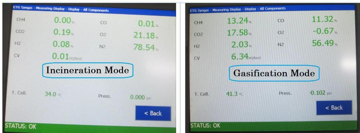
**Safe emission in Incineration mode and good syngas quality in gasification mode**
