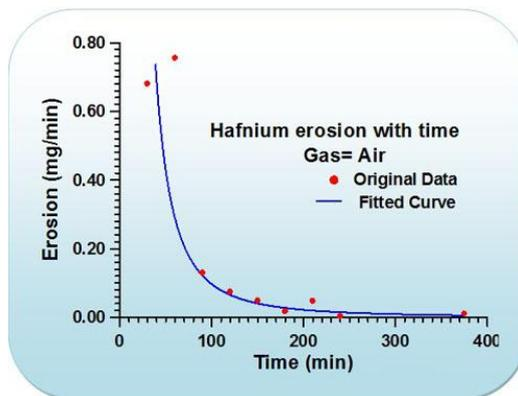
As shown above extremely low electrode loss due to erosion is observed for the cathodes. For new electrodes, the loss is relatively high at the start but decreases fast with time and stays at that extremely low level. The electrode loss reduces with increase in current.
