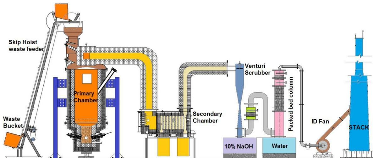
**Components of Triple Torch Air Plasma Incinerator**
