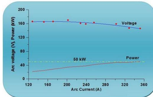
Typical V-I characteristics for the plasma torch is shown in figure above. The arc voltage remains nearly constant over a range of currents. A slight drop in the voltage is observed at higher currents. Increase in power with increase in current is slightly non-linear. For operation around 50 kW the torch operates near current 350 A and voltage 156 V.
