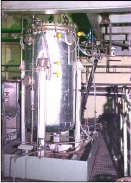
**Test Facility for Passive Containment Cooling system**
