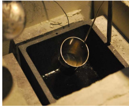
Graphite crucible containing molten fluoride salts
