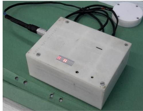
External Interface Unit (EIU) for programming & charging of IPG, with wireless interface with IPG & PP/CP.
