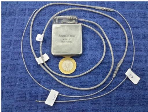
Implantable components: Pulse Generator (IPG), Brain Lead, Intermediate Lead
