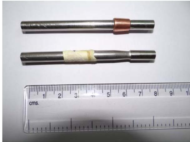
Fig.5.13 Joined samples of the D9 clad to SS316L end plug
