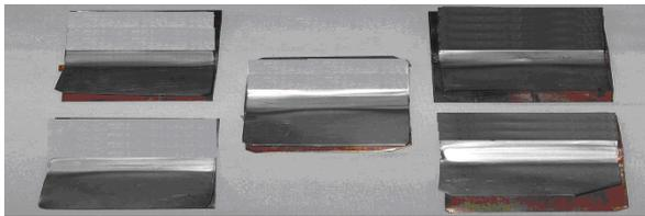
**Fig 5.9 Cu -SS sheets EM Welded Samples welds**
