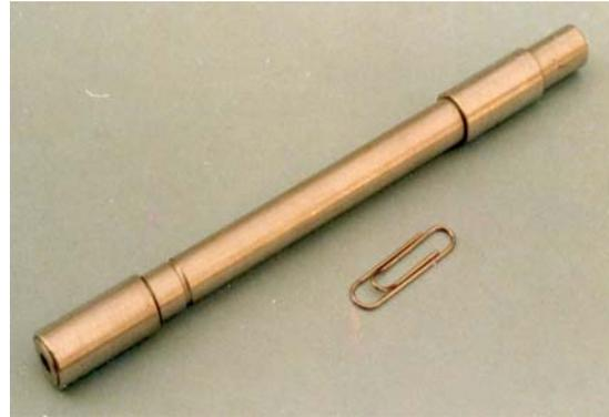
**Fig 5.1 Magnetic Flux Concentrator** **Fig 5.2 Two Al plugs collapsed at two ends of Al rod**
