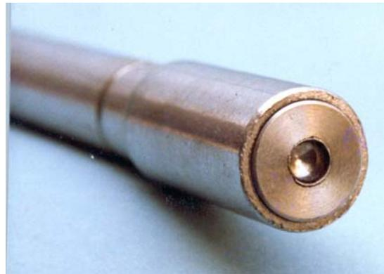
**Fig 5.3 Copper lug swaged on Al-multi-core cable** **Fig 5. 4 Al-plug collapsed on SS-rod**
