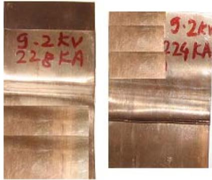
**Fig 5.8 Cu -Cu sheets EM welded**
