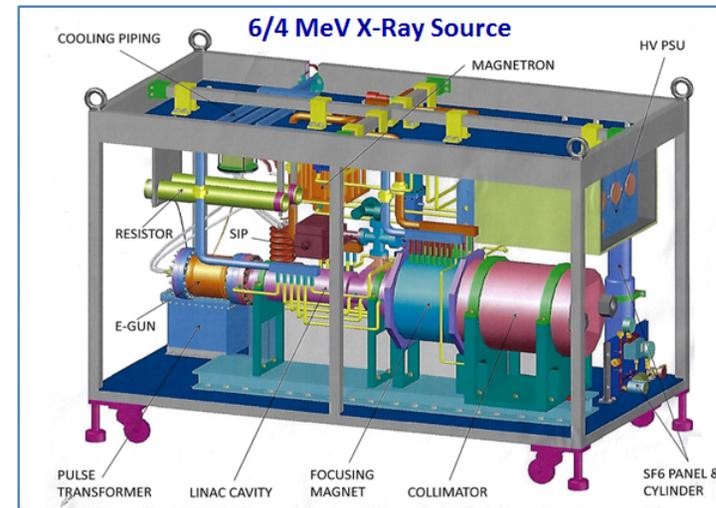
6/4 MeV Portal Single Energy Cargo Scanner System & 3-D Model of the X-Ray Source
