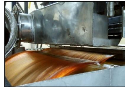
Effluent flow under electron beam
