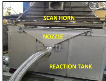
Reaction tank and nozzle in beam room
