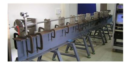
SHPB is an inhouse developed experimental test setup that is used to evaluate material property at high strain rate loading. The data generated is used for design and safety analysis of impact events such as 9 m drop test of radio-active material shipping cask. This setup is used to carry out compression and tensile tests in strain rate range of  $10^2$  to  $10^4$  s<sup>-1</sup>.
