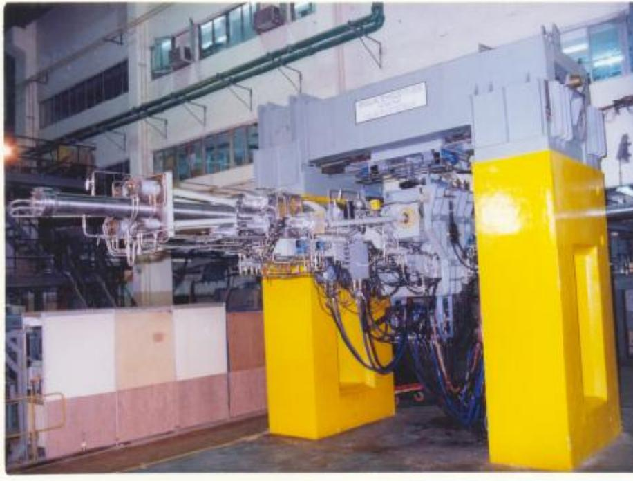
**FM HEAD & TEST CARRIAGE OF 540 MWe PHWR AT ENGG HALL-7, RTD, BARC**
