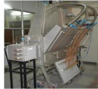
The schematic of the channel disassembly test facility
