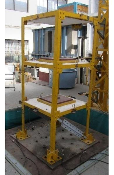
Shake Table Testing of Steel Frame with BRB
