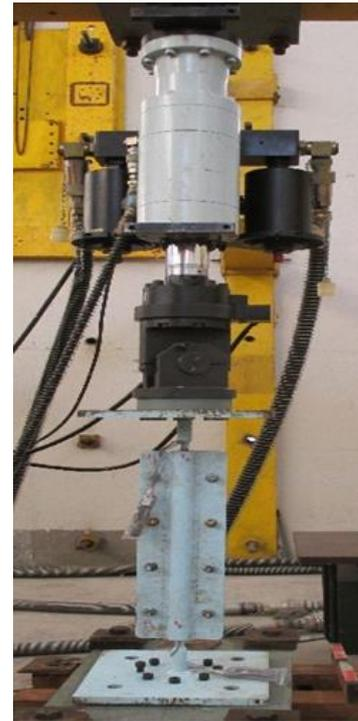
Buckling Restrained Bracing (BRB)
