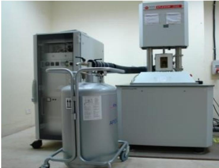
*DMA is currently used to determine mechanical properties using small scale specimen tests on various types of specimens of metals and alloys under static and dynamic loads.*
