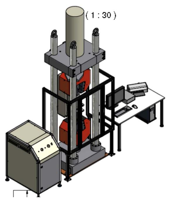
Universal Testing Machine(UTM) is used to characterize the properties of steel like Young's modulus, Ultimate strength, yield stress, ductility etc. It is used to evaluate the tensile capacity of various specimens. Plate specimen and round bar specimens can be tested in the machine. The machine is located at ground floor, Hall 11. The capacity of the machine is 1200kN.
