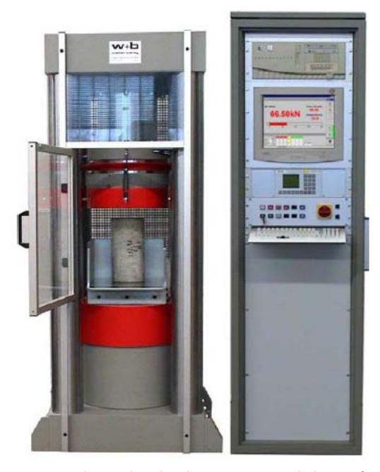
Compression Testing machine is used to evaluate the maximum compressive load capacity of concrete cubes or cylinders. It is mainly used to assess the grade of concrete. It can also be used to evaluate the Young's modulus of concrete cylinder. The machine is located at ground floor, Hall 11. The capacity of the machine is 3000kN.
