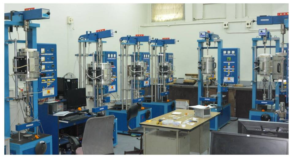
Creep testing up to 1000 °C
