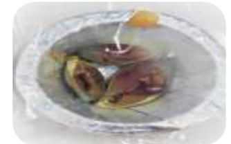
Change in color indicator dot based on beetroot extract in packaging film due to spoilage of fish
