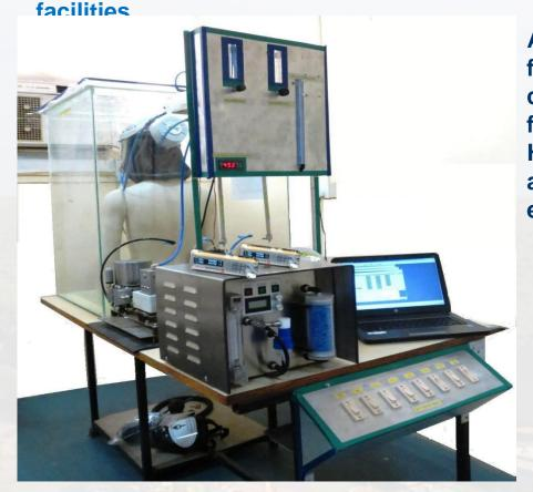
A test facility has also been established to test various filter media for their filtration efficiency and pressure drop against airborne radioactive contaminants in nuclear facilities. The filter media such as micro glass fiber filter media for HEPA filter, HEPA plus carbon granules filter media, HEPA cartridge filter media, electrostatic filter media, microdot filter media and disposable masks can be tested using this facility for their filtration efficiency and pressure drop.
