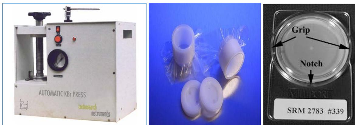
Fig: Pellet making Machine
