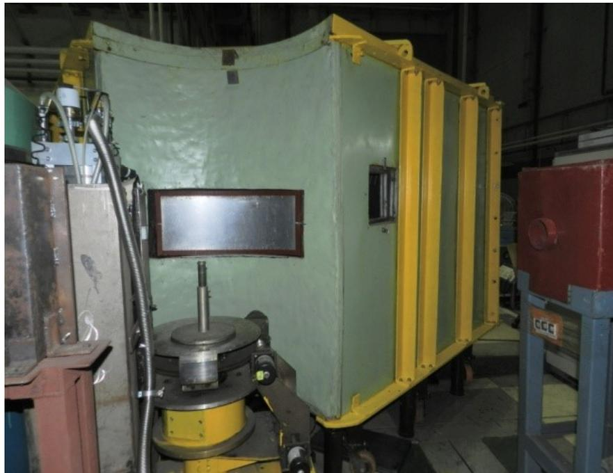
For measurements of phonon density of states, crystal field excitations, and quasielastic scattering.
