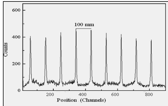
Position spectrum of a  $^3\text{He}$  PSD with slit-3 and 10 cm spacing
