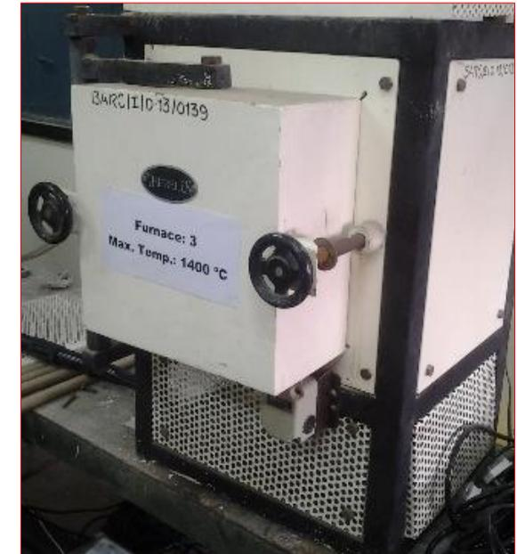
Electrical heating furnace with ambient condition suitable for preparing oxide sample
