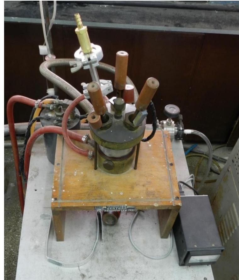
**Arc Melting is used to prepare alloy samples.**
