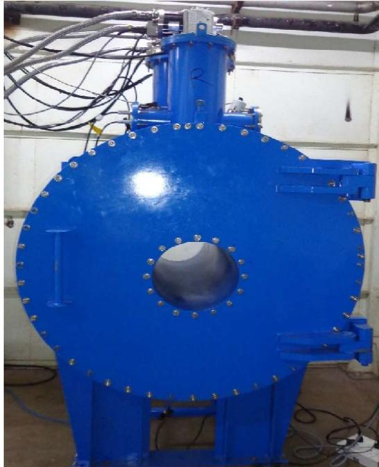
300mm diameter Warm bore superconducting solenoid magnet
