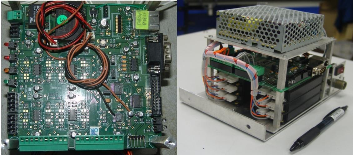
**Brief Description:** Compact zoom lens electronics (with up to 8 no. highly protected 0 to 2KV zoom lens and DCQ supplies) has been developed to steer the ion beam after analyser towards the collector cup.
