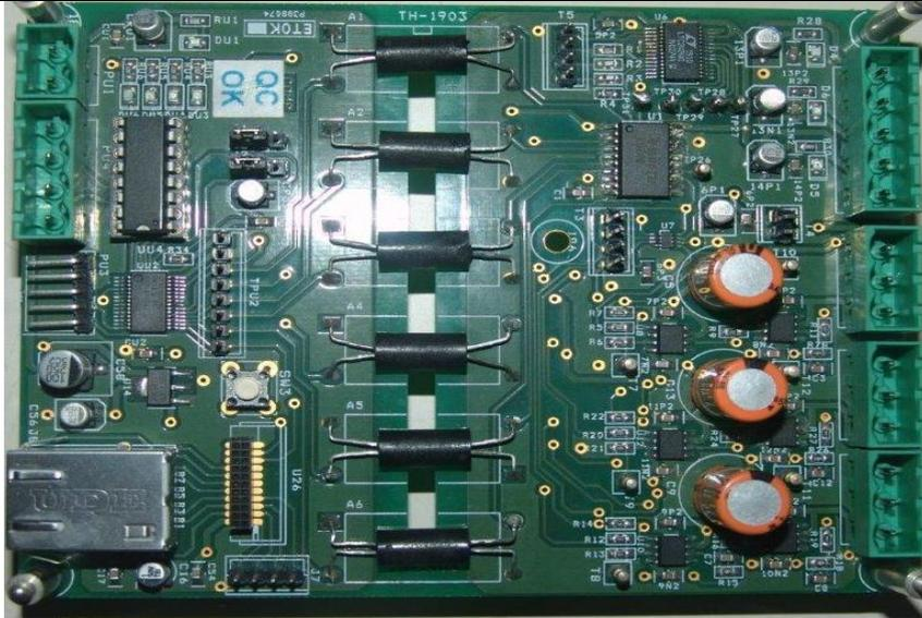
**Brief Description:** This card has been used to control triple filament assembly of Thermal Ionisation Mass Spectrometer (TIMS). It consists of SoC controller, dual DAC, OP AMP based IGBT driver, 10 kV optical isolators, Ethernet controller etc.
