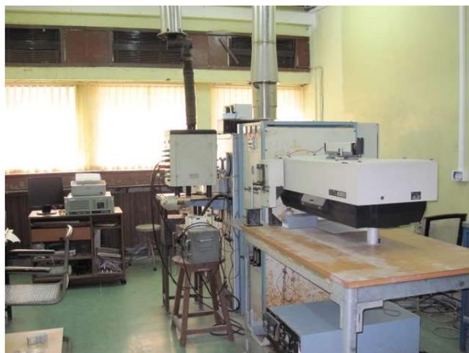
Fig. 1. DC Arc Atomic Emission Spectrometer
