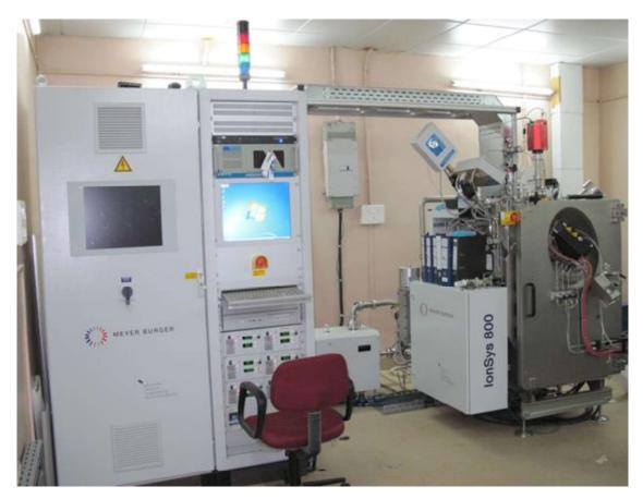
• State-of-art Dual Ion Beam Sputtering system
