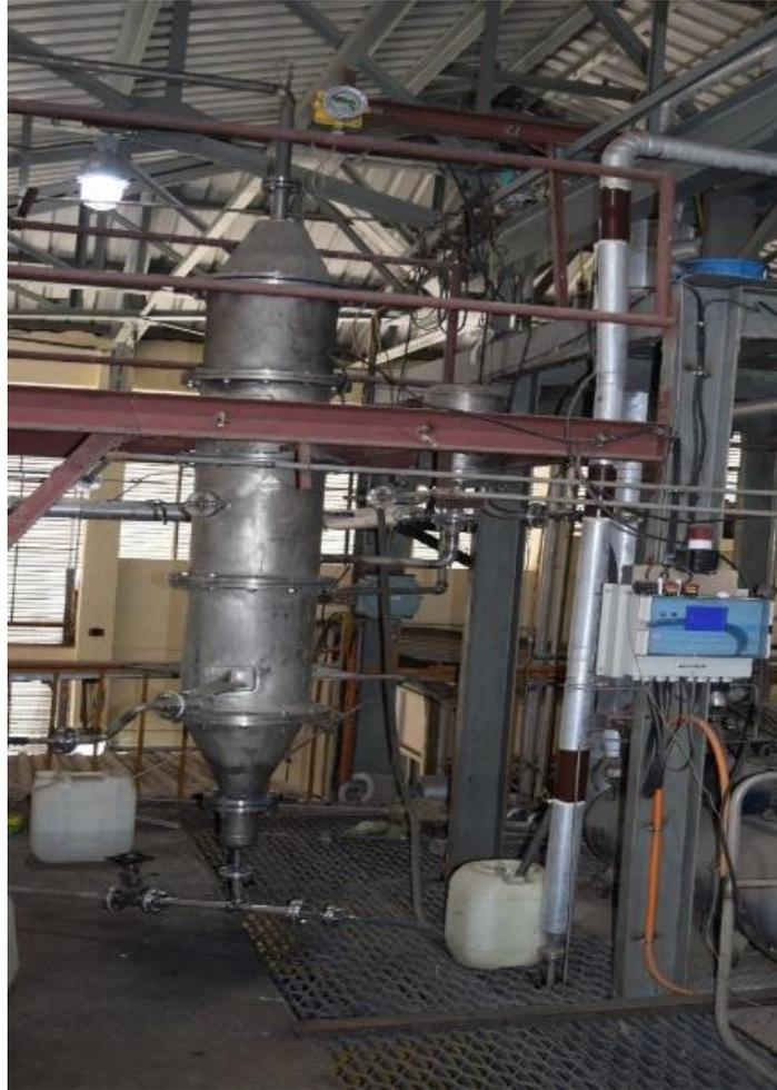
Fig.4 Multi-stage circulating fluidized bed (MSCFB) for organic vapour adsorption, recovery and reuse.
