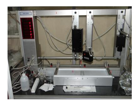
•This system allows to deposit thin films by LB technique, which provides highly ordered thin films of various organic materials based on amphiphilic molecules.
