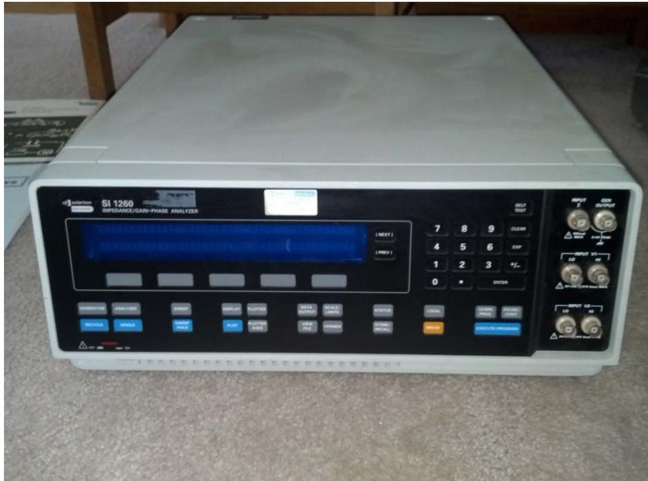
The instrument measures impedance of solid and liquid samples in the frequency range 1  $\mu$ Hz to 32 MHz. A high temperature cell has been attached to this instrument to measure the conductivity, dielectric constant of solid samples up to 800  $^{\circ}$ C.
