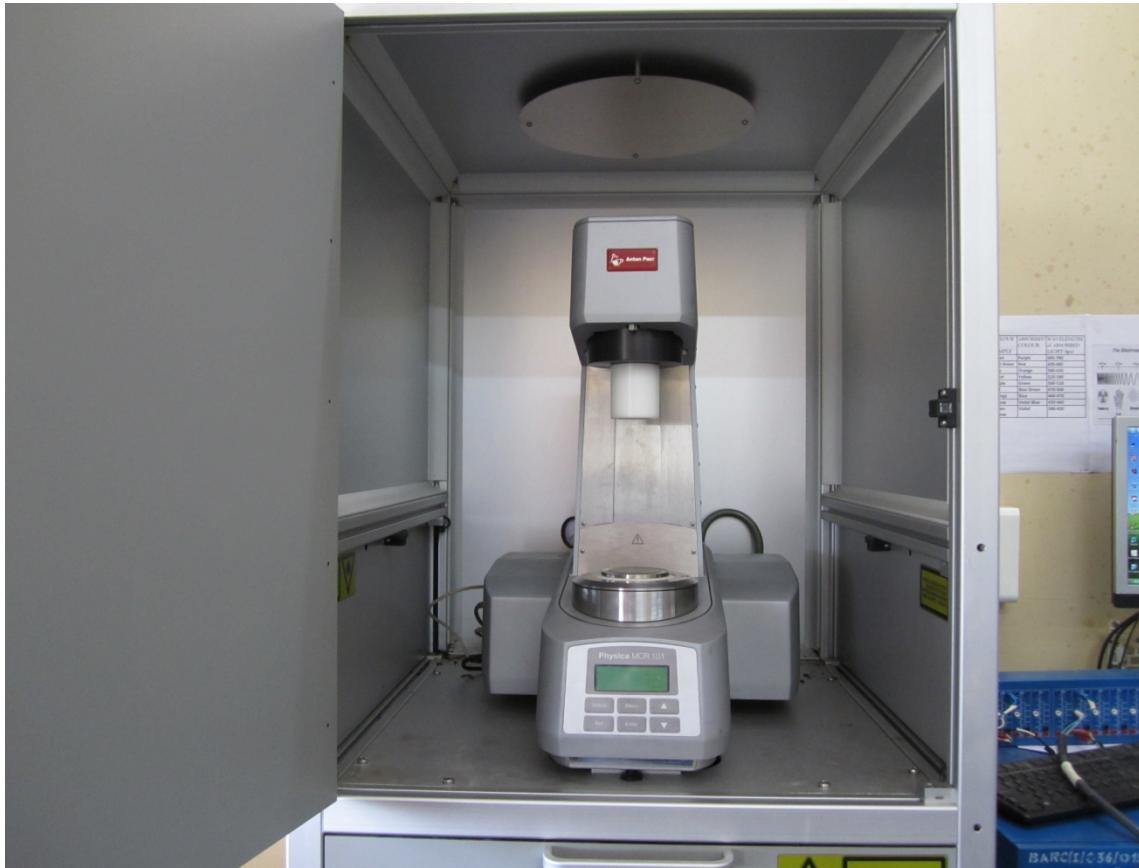
Used to characterise rheological parameters (viscosity, shear modulus etc) of complex fluids
