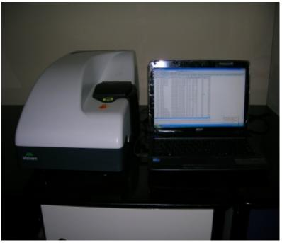
Useful to characterise nanoparticle size and surface charge.
