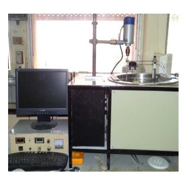
Measures enthalpy change accompanying dissolution of oxides, alloys in a known solvent. The instrument gives useful data on standard molar enthalpy of formation of compounds.
