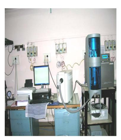
Used to measure mass changes of decomposition reactions as a function of temperature. It can be also be used
