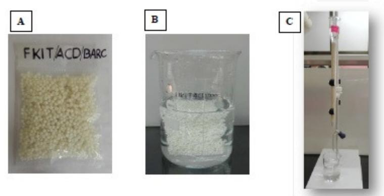
(A) Kit for decontamination of fluoride from groundwater (B) for batch method; (C) for column method
