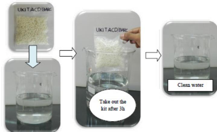
Decontamination of U from groundwater in field condition in batch method
