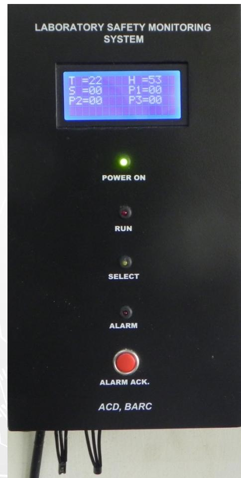
Compact controller unit with local display, audio visual alarm and Temperature, humidity and smoke sensors deployed in each laboratory
