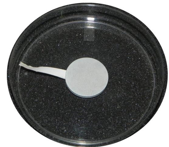
Cd deposition at 200  $\mu\text{m}$
