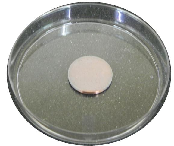
Cd deposition at 100  $\mu\text{m}$
