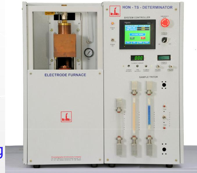
**Principle :** The equipment is based on inert gas fusion technique. The sample is heated to a high temperature in a graphite crucible with tin flux under inert atmosphere. Hydrogen is detected by thermal conductivity detector
