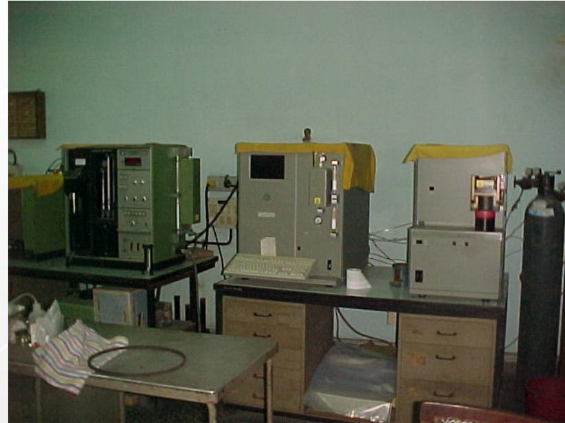
**Principle:** The sample is heated to a high temperature in a graphite crucible with or without nickel flux depending upon the specimen under inert atmosphere. Oxygen is detected as carbon di-oxide by IR detector and nitrogen by thermal conductivity detector.
