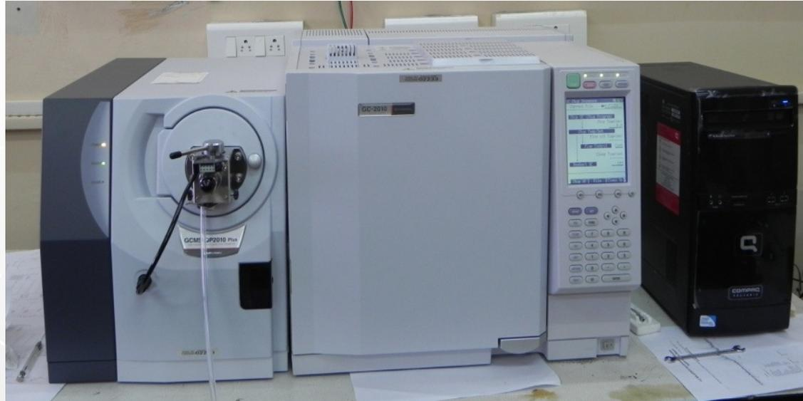
**Applications** : Identification and quantification of volatile and semi volatile organic compounds in complex mixtures eg. pesticides in food, beverages, organic pollutants in water, environmental samples, etc.
