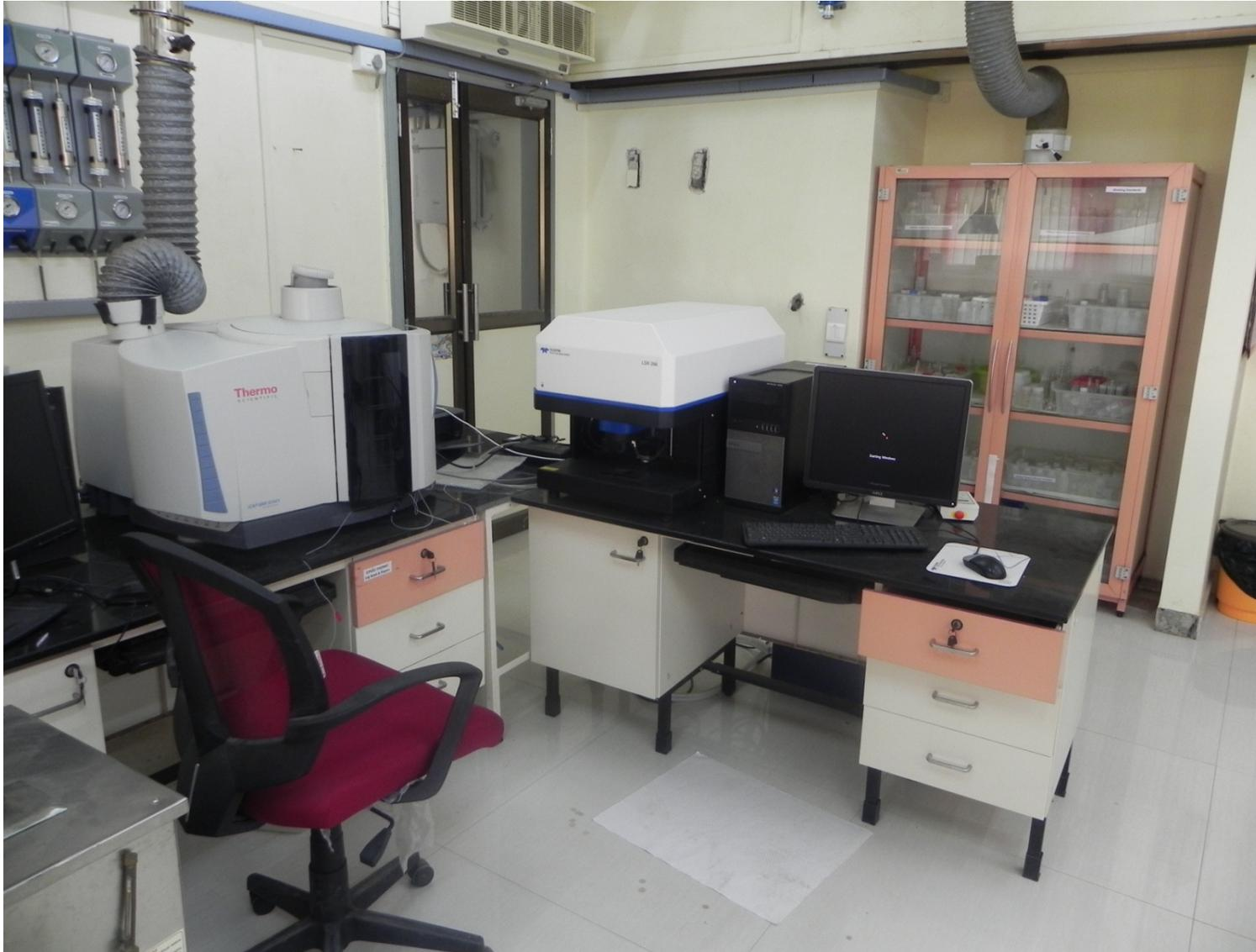
**Inductively coupled plasma–optical emission spectrometer coupled with laser ablation system : For analysis of trace elements in metals and rock samples.**
