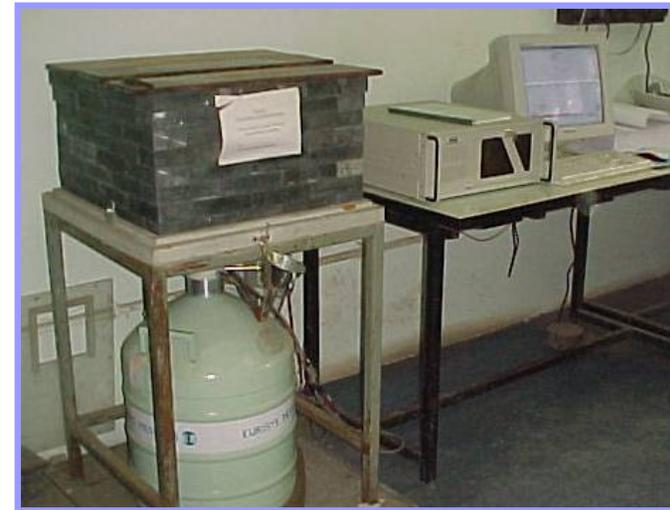
Characteristic gamma radiations emitted from radio nuclides are measured using HPGe detector. Intensity of gamma radiations are proportional to the concentration of radio nuclides
