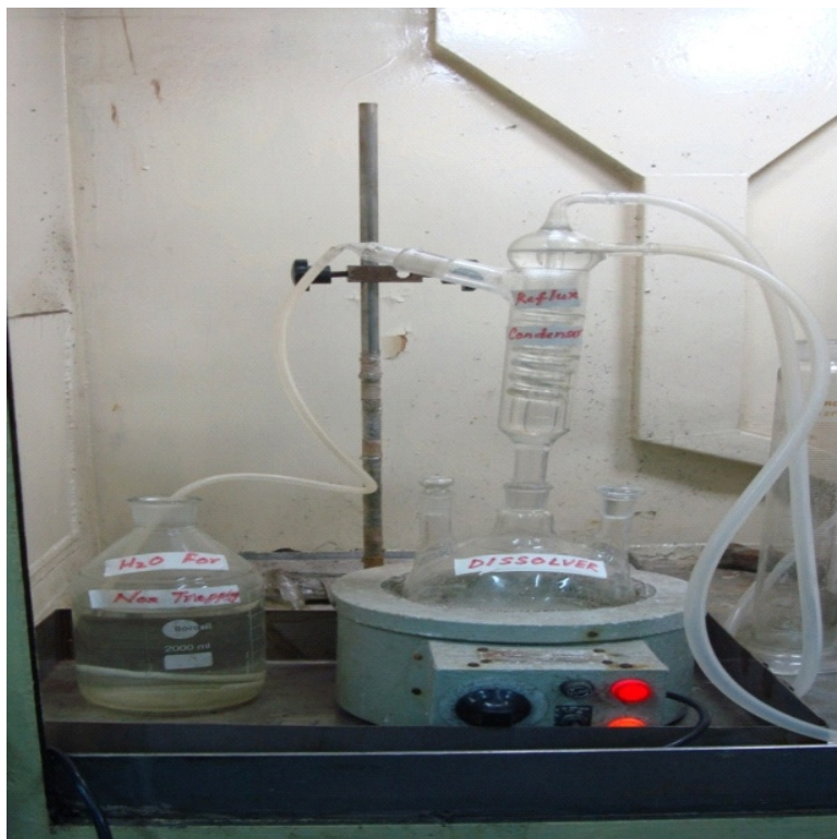
Dissolution setup for Al 6061.
