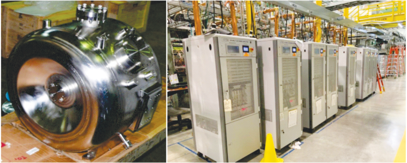
SC-Single Spoke Resonator and 7 kW Solid State Power Amplifier systems: Other in-kind contributions of India to FNAL.
