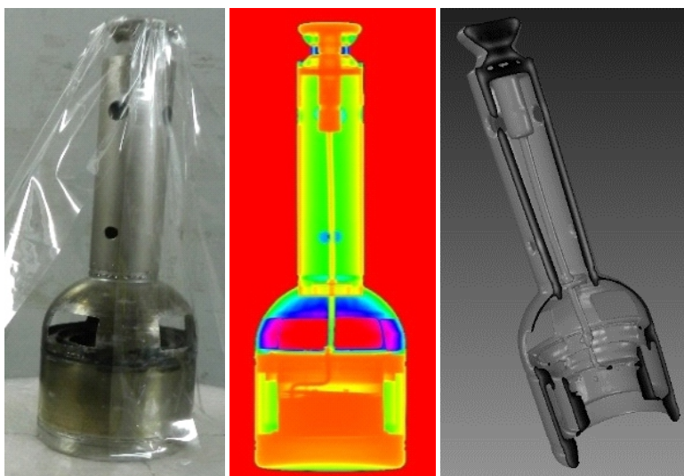
Cathode ray assembly, Digital radiograph and Volume CT image.
