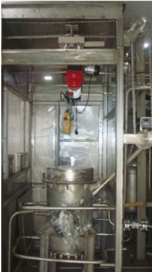
Pilot scale experimental setup for remote handling of unirradiated simulated SUPF.
