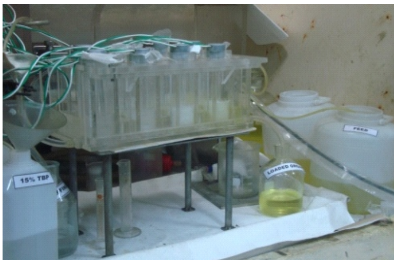
Laboratory scale mixer-settler for recovery and decontamination of U.
