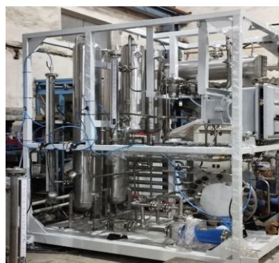
Fig.4: 150 kW Alkaline water electrolyser plant developed under incubation.
