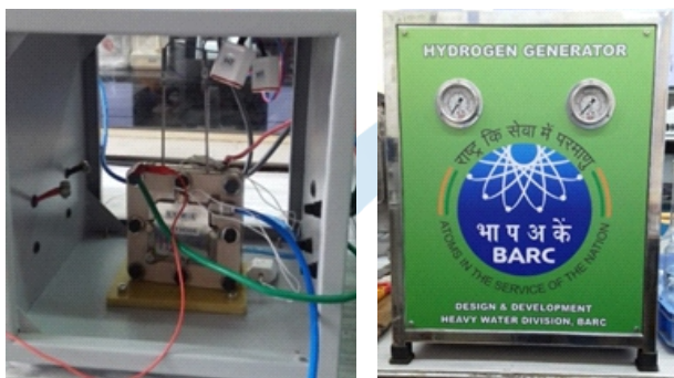
Fig.9: Indegenous PEM cell stack and PEM based laboratory hydrogen generator.
