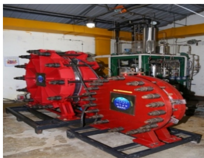
Fig.5: Prototype 0.5 MW and 1 MW Alkaline water electrolyser stacks under testing at BARC.
