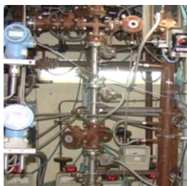
I-S Thermochemical cycle for H_2 production: Bunsen reactor in Metallic Bunsen setup.
