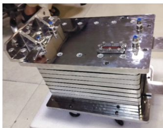
AWE Tech. for H_2 production: Scaled up 10 Cell capillary electrolyser stack.
