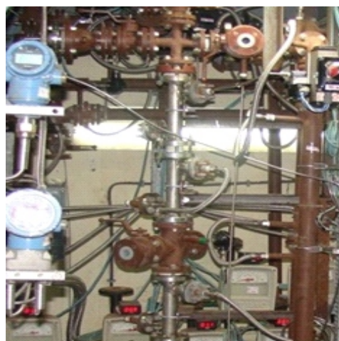
Fig.6: Bunsen reactor in Metallic Bunsen setup.
