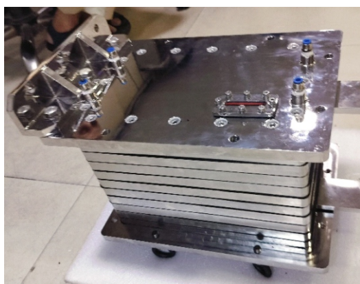
Fig. 7: Scaled up 10 Cell capillary electrolyser stack.
