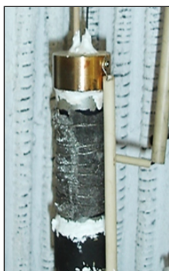
Fig.6: Single Cell Tubular HTSE during long-term testing.
