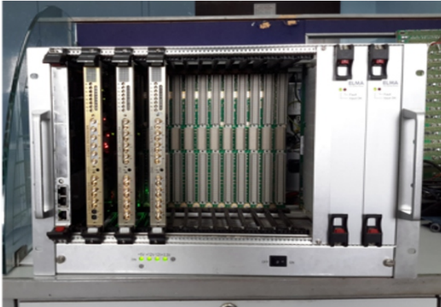
Fig. 10: VME64x based RF Protection Interlock System.
