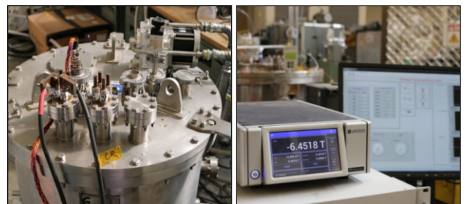
Fig.8: Cryostat housing the conduction cooled magnet assembly during cryogenics tests & the measured magnetic field in the aperture @ 43.5A.
