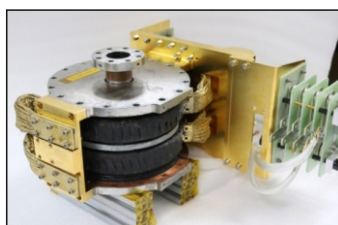
Dressed magnet assembly with heat sinks and cold diodes
