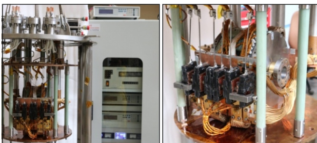
Fig.7: Magnet assembly integrated with indigenous cryo-cooler based magnet test stand.
