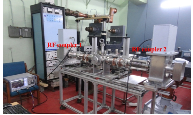
Fig.10: The 650 MHz high-power test facility setup, featuring a central cavity positioned between two prototype couplers for standing wave mode evaluation.
