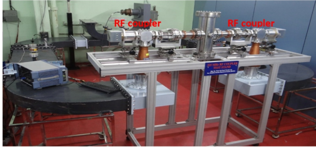
Fig.8: The high-power 325 MHz resonant ring test stand with two integrated prototype couplers undergoing testing.
