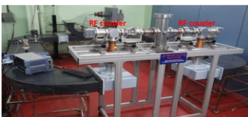
The high-power 325 MHz resonant ring test stand with two integrated prototype couplers undergoing testing
