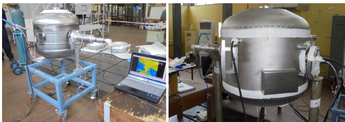
Fig.16: Bare Cavity preparation for Jacketing and Jacketing of Bare Cavity.
