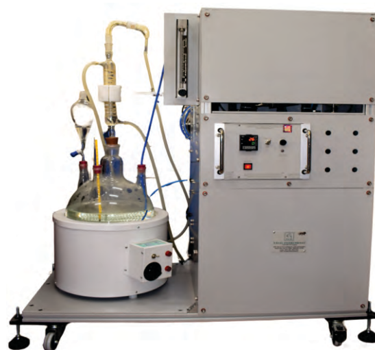
The Wet-Oxidizer system for extraction of dissolved inorganic and organic species of C-14 in liquid samples.
