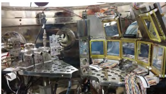
Silicon strip detector array at the BARC-TIFR Pelletron Linac Facility.
