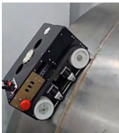
Robotic crawlers designed for examining stainless steel and nonmagnetic structures.
