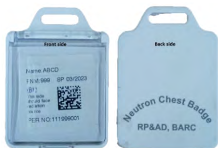
Front and Back sides of Chest Neutron dosimeter developed in BARC.
