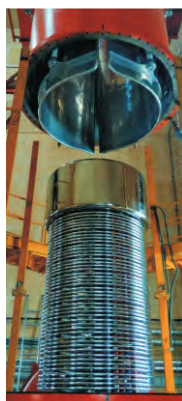
Electron Beam accelerator for wastewater treatment(Right).
