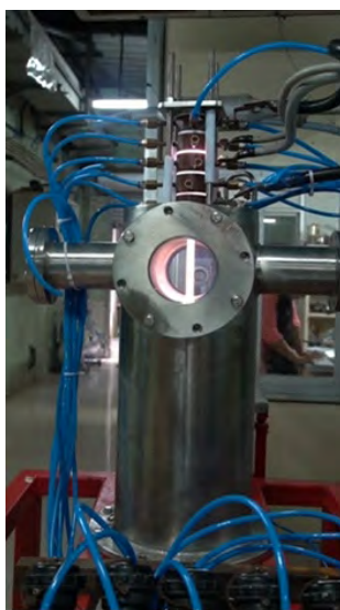
Non-divergent stable Helium thermal plasma.
