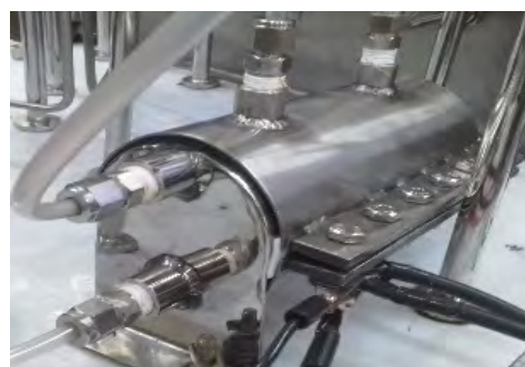
Cell for laboratory H_2 generator.
