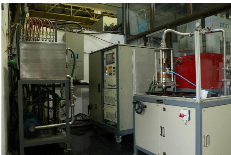
Fig.3: Induction Levitation Melter installed at Modular Laboratory, BARC.
